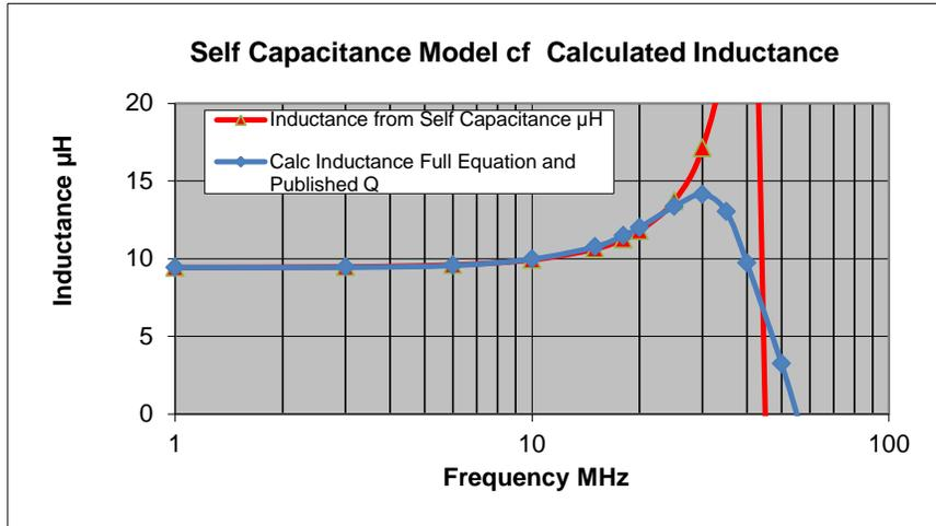
Figure 7.2.1 Self Capacitance Model and Measured Inductance Matl 61
