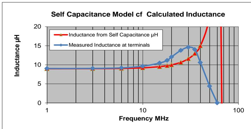
Figure 6.2 Self Capacitance Model cf Measured Inductance
