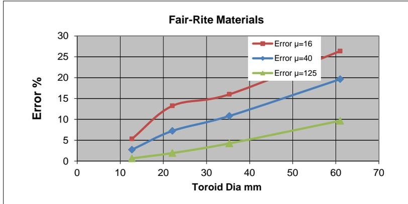
Figure 20.1 Error for  $N=5$ , irrespective of core diameter
