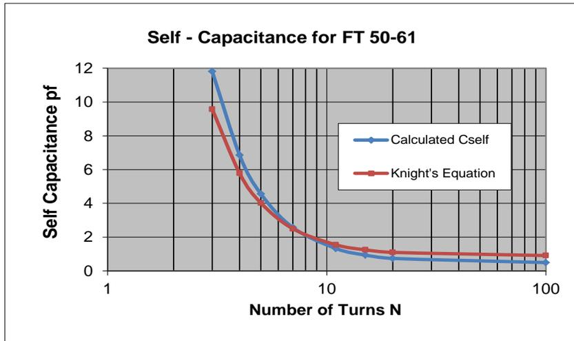
Figure 16.1 Comparison of Theory with Knight's measurements
