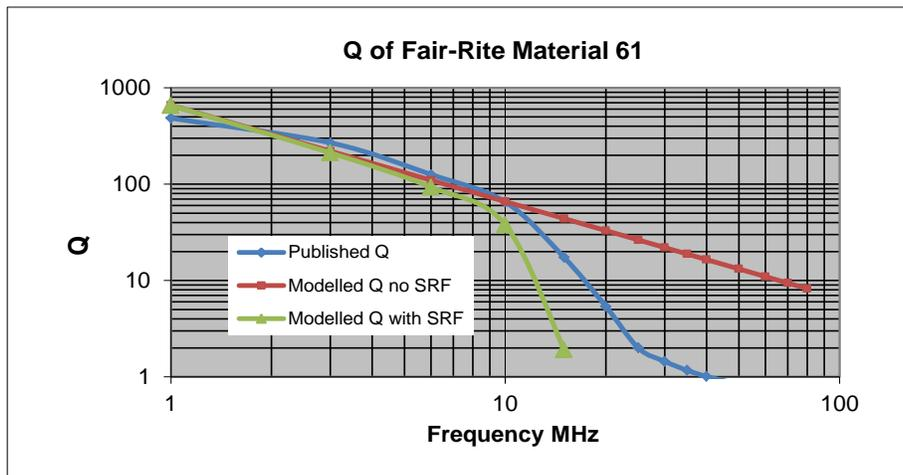
Figure 8.1.4 Modelled Q with effects of SRF (Material 61)
