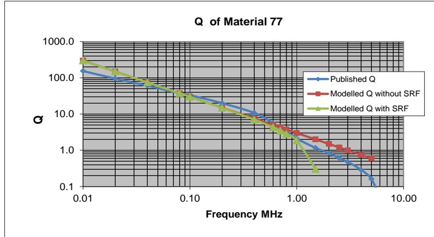
Figure 8.1.5 Modelled Q with effect of SRF (Material 77)
