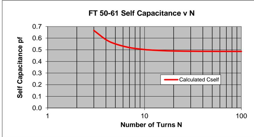
Figure 6.1 Calculated Self Capacitance of FT50-61 core
