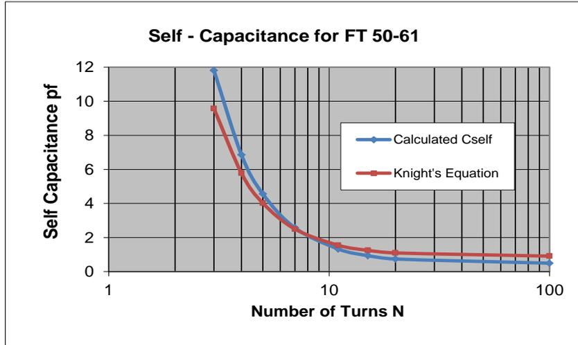
Figure 2.1 Comparison of Theory with Knight's measurements
