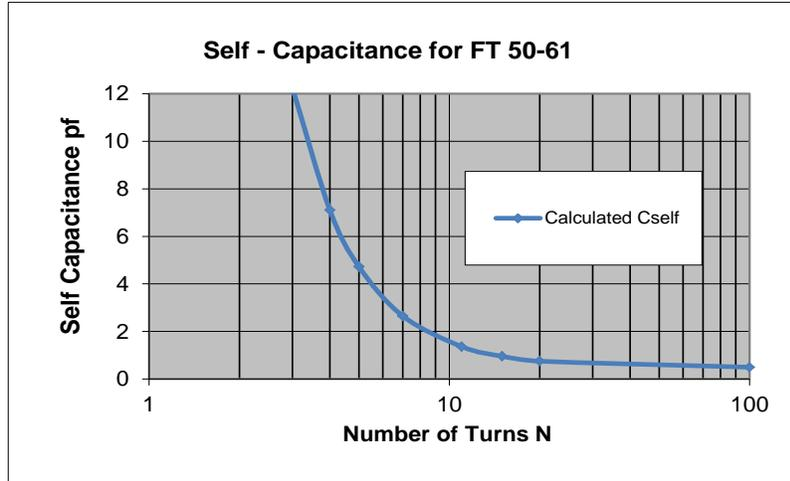
Figure 7.2.2 Self Capacitance Model for FT 50-61
