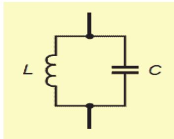
Figure 5.1 Equivalent circuit for self-resonance
