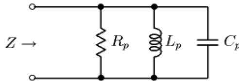
Figure 8.1.2 Self-capacitance model with Loss
