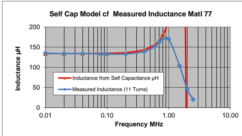
Figure 7.2.3 Self Capacitance Model and Measured Inductance Material 77
