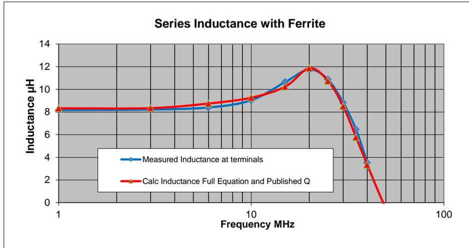
Figure 10.1 Comparison of Theory with Measurements (full equations)
