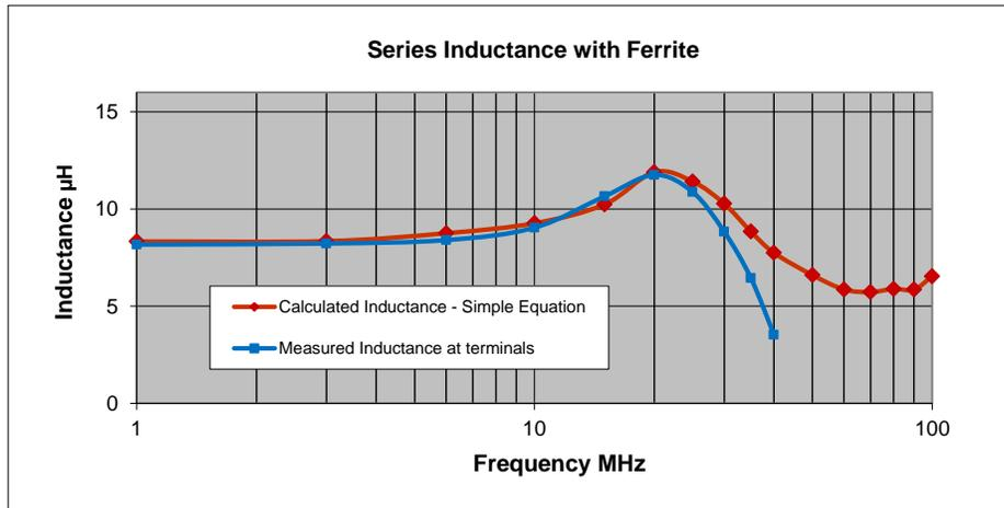
Figure 10.2 Comparison of Theory with Measurements (simple equations)
