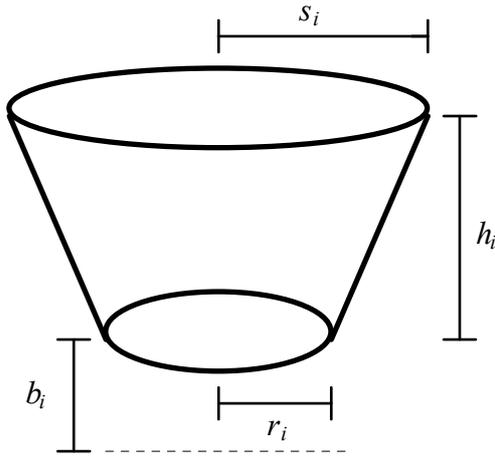
Fig. 1. Conical coil.
